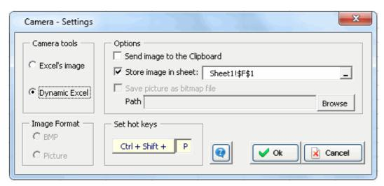
Select a range as shown in the example and click the Camera icon The range is copied as a dynamic image in the target cell selected, F2 in this example. Any changes in the source range will be reflected in the target image.
